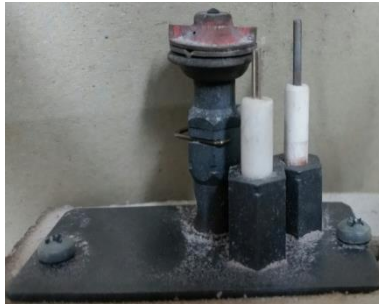
Pilot with bracket, hood, injector,spark and flame sensor
